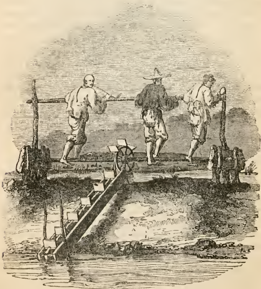
Chain pump. From Staunton.
